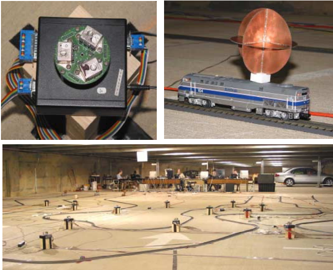
Fig. 1. Sensor Network. Top left: radar unit with three sensing heads. Top right: vehicle being tracked. Bottom: an example configuration with 35 sensors and 3 vehicles
