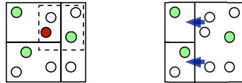
Figure 7 - Dynamic partitions, either roaming (left) or resizable (right).
