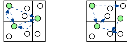
Figure 6 - Control-permeable partitions, either manager directed (left) or sensor directed (right).
